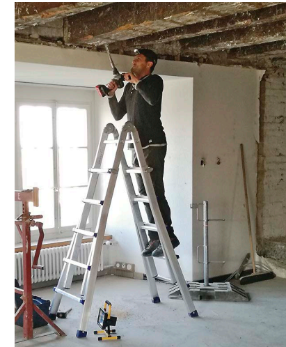
Wood sampling in Burgdorf Castle. The trees for the massive ceiling beams of spruce and silver fir were felled in 1200 AD, worked into shape and probably used shortly afterwards.
